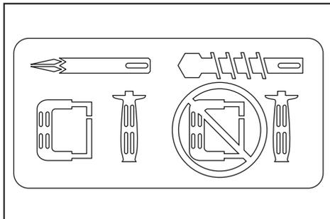
**CAUTION:** Use the side handle only when chipping, scaling or demolishing. Do not use it when drilling in concrete, masonry, etc. The tool cannot be held properly with this side handle when drilling.
