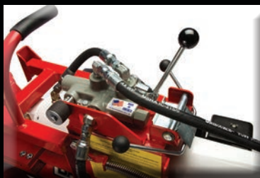
Two handed control provides operational safety
