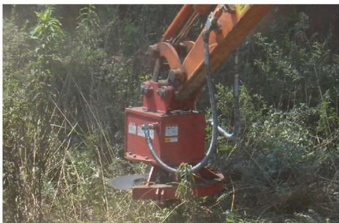
3. Blade for hard grass / bamboo Teeth : 100pcs
