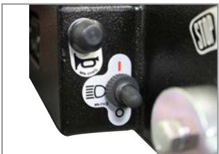
Horn and headlight switch for job-site safety
