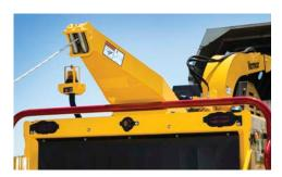
**EASILY LIFT HEAVY MATERIAL.** An optional winch allows operators to move large logs effortlessly. The 150' (45.7 m) winch line has 2000 lb (907.2 kg) pulling force and can automatically lift the log onto the feed table. With the chain choker detached is it also more easily attached to log than hook-on cable designs.
