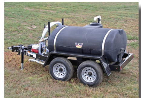
500 Gallon “Express” Potable Water Trailer (non-certified) All components of this non-certified trailer are rated for potable water.
